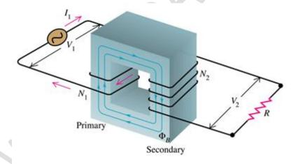
A transformer consists of rectangular soft iron core made of laminated sheets, well insulated from one another.
