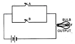
In this arrangement, off (or open) corresponds to 0 and on (or closed) corresponds to 1. The inputs are introduce through the switch A and B. The lighting of the bulb is the output. Here we find that the bulb glows (i.e. output is 1) when either switch A is closed or B is closed or both the switches are closed. The bulb remains off (i.e. output is 0) only when both the switches A and B are open
